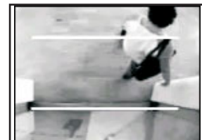
An example from a video clip showing the two detection zone markers.
